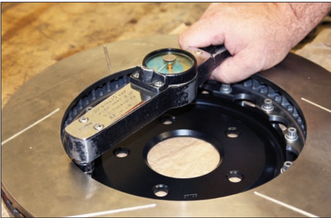
Sequence 8: Using an alternating sequence, torque bolts to 155 in-lbs.
