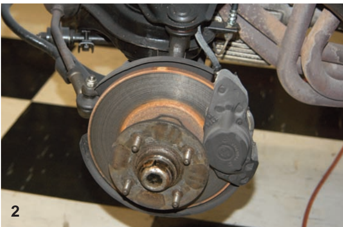
The original brakes used a single piston caliper and a small 10-inch diameter solid rotor. The brakes were adequate for standard driving with a 260 engine but certainly not enough for this car that sees track action with a very hot Ford 302ci engine.
