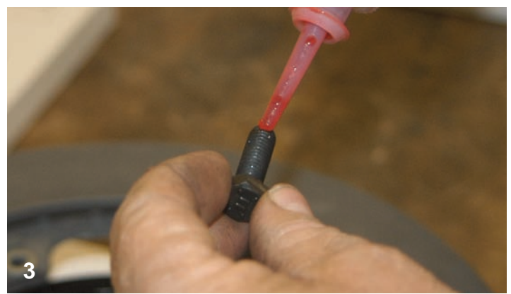
The Wilwood rotor has to be bolted to the aluminum hub assembly. Here the bolts are being coated with Loctite 271.
