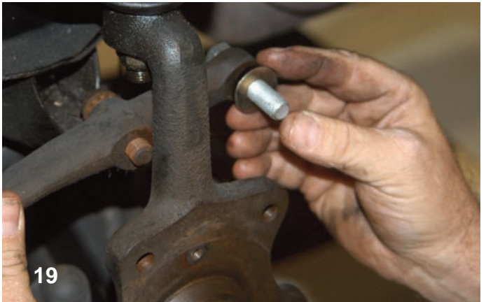
19 The bolt that connects the bracket to the spindle was loaded with a spacer and a shim washer.
