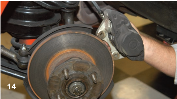
14 After the caliper bolts were disconnected, the caliper could be removed from the disc brake assembly.
