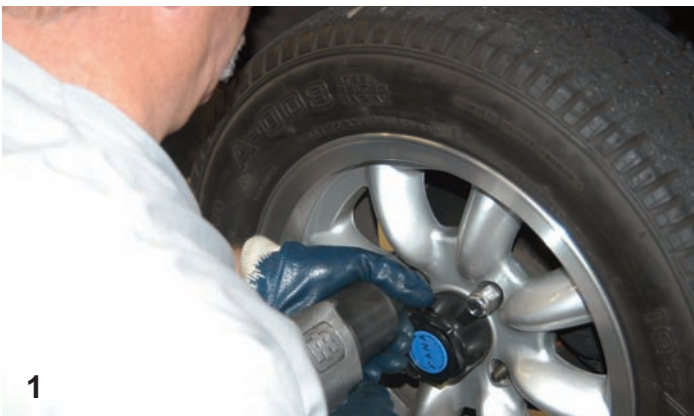
Using an impact gun and the appropriate size socket, the four lug nuts were disconnected and then the wheels and tires were removed from the car.
