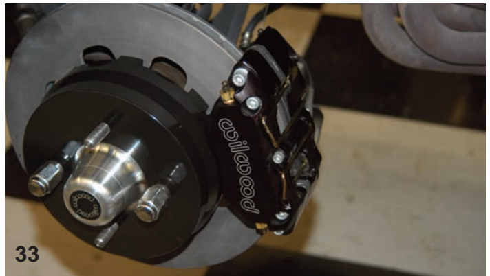
Here is the finished brake assembly using a Dynapro Caliper and an 11.75-inch rotor assembly. This should provide ample stopping power for the hot Tiger.
