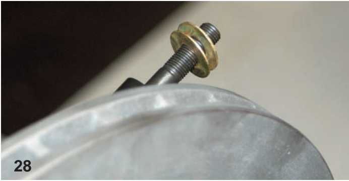
The caliper bracket stud was loaded with two shim washers.
