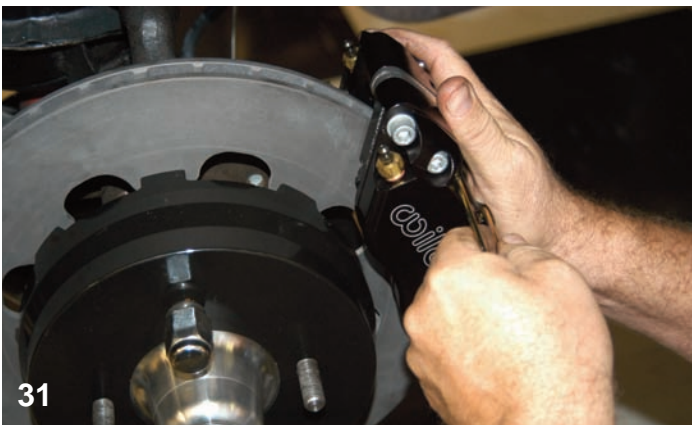
After the brake pads were in place, the spring-loaded retainer clip was installed.
