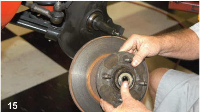
15 After the caliper was disconnected, the rotor assembly could be removed from the car.
