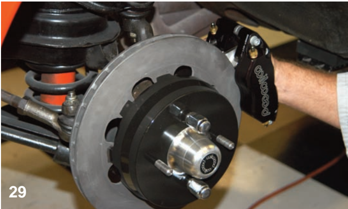
The caliper was placed over the rotor and then the caliper was aligned over the two mounting studs. The caliper was centered over the rotor assembly.
