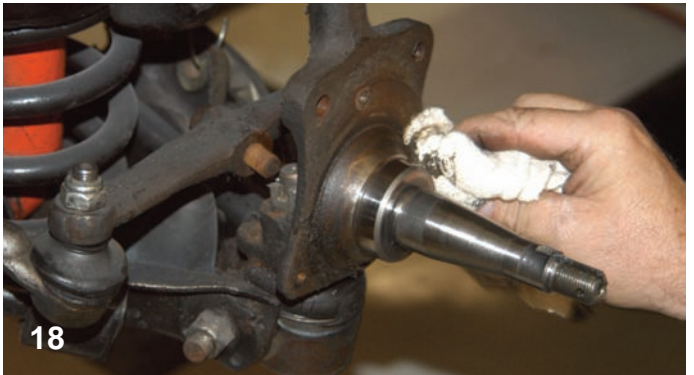
18 After the dust shield was removed, the spindle was cleaned off using a rag and cleaning solvent.
