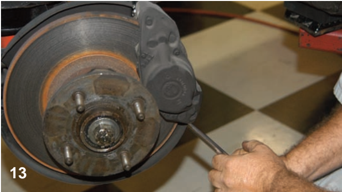
13 The caliper is held on with two bolts. Here the bolts are being broken loose with a large breaker bar. After the bolts are loose they can be removed with a ratchet wrench.
