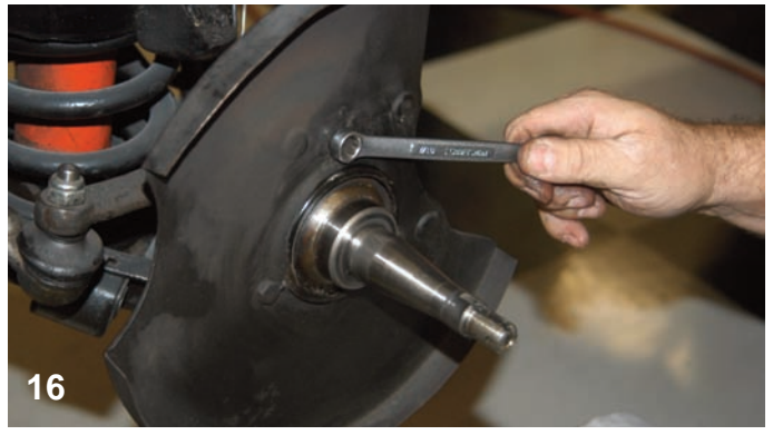
16 After the rotor was removed, the small bolts that secure the dust shield to the spindle assembly could be disconnected.
