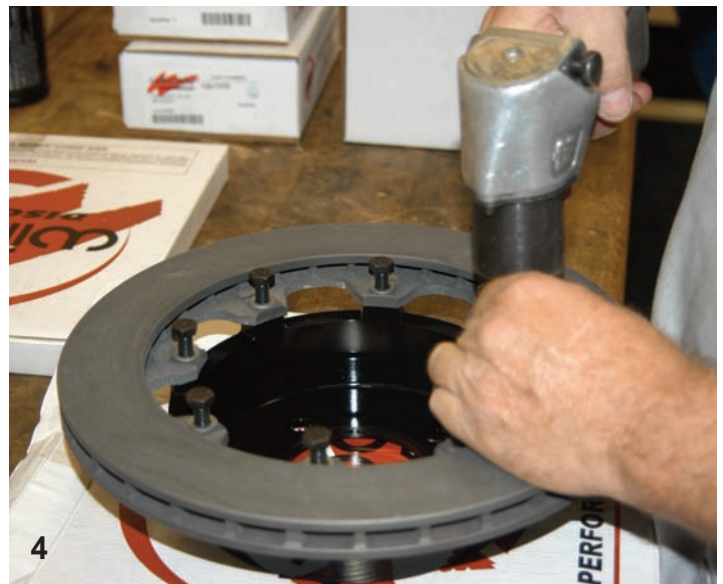
The bolts were screwed into the hub assembly finger tight. Notice each bolt uses a small flat washer.
