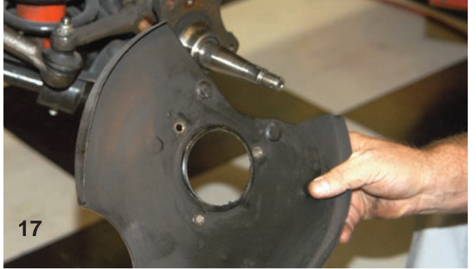
17 The dust shield was removed from the spindle to provide more clearance for the larger rotor.
