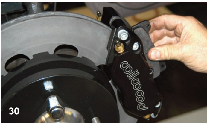
The BP-10 Smart Pads were installed in the caliper making sure they are all the way in..
