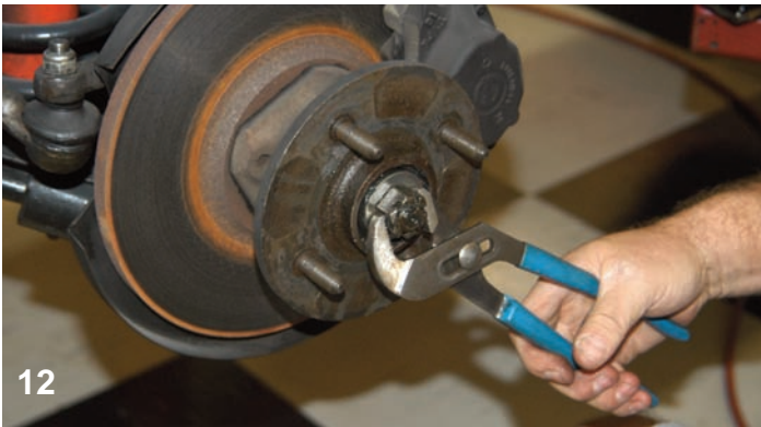
12 The cotter key was removed and then the spindle nut was disconnected from the spindle using channel lock pliers.
