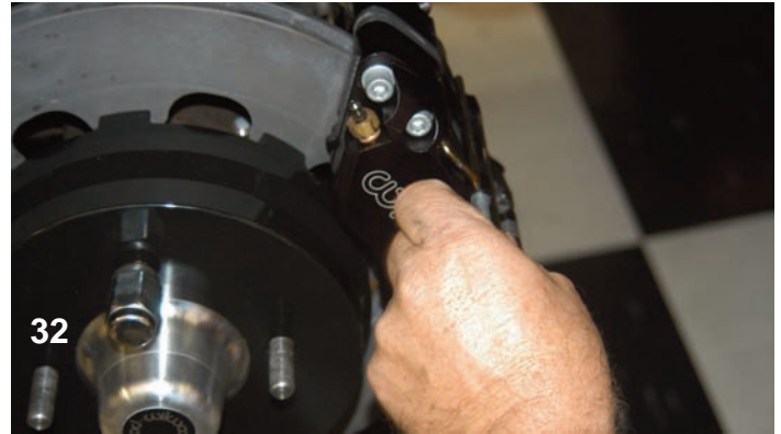
After the retainer clip was installed, the bridge bolt and tube could be installed and tightened.
