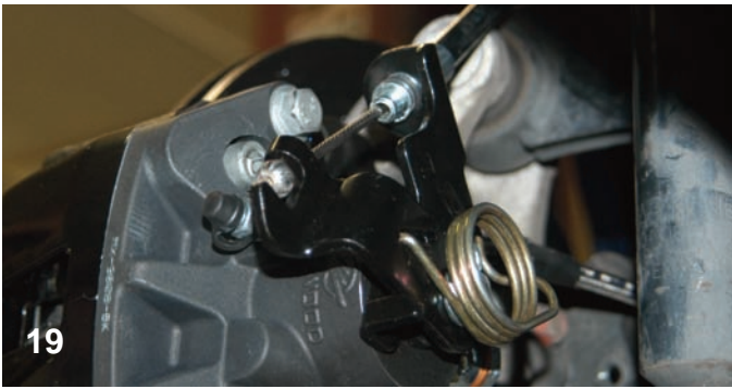
The other end of the cable fits through the bracket hole and the cable end fits into the mechanism lever. When the lever is pulled back the parking brake is applied.
