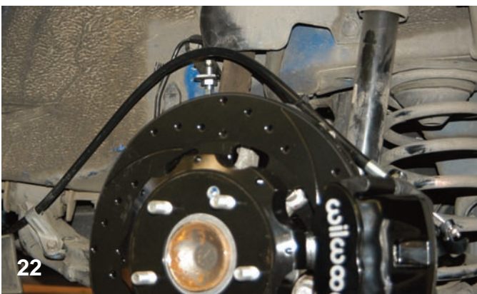
The cable is held at the front with an original bracket and then it runs to the caliper bracket. A small plastic tie wrap is used to keep the cable in place as it crosses over to the caliper.
