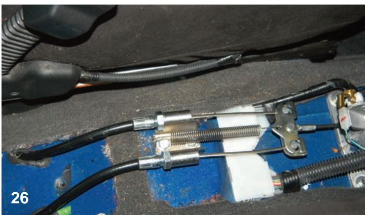
Looking inside of the car you can see the two cables routed perfectly into the original Honda brackets. This looks like a factory installation.
