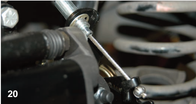
A close look reveals the C-clip that holds the cable end securely in the bracket.
