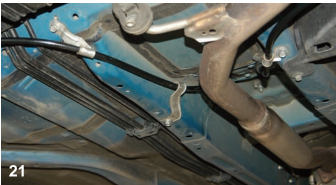
Looking under the car you can see the cable being routed from the inside of the car back along the undercarriage. The original cable brackets work great with the new cable.
