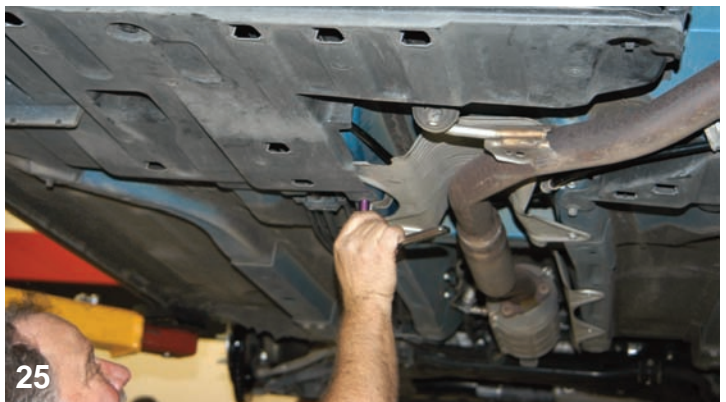
The front of the plastic panel was secured with the original sheet metal bolts.
