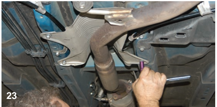
The exhaust heat shield was reinstalled and the bolts were secured with a socket wrench and the correct size socket.
