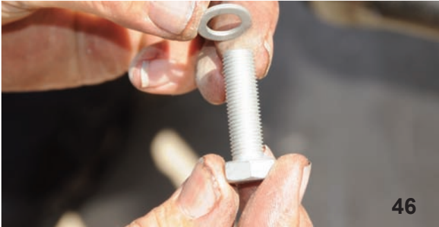
A washer was installed on the caliper bolt and then the bolt was coated with Loctite.
