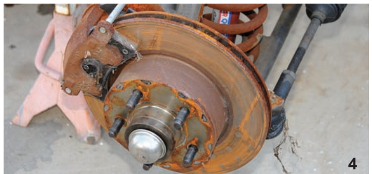
This chassis is running a Total Cost Involved Engineering economy front suspension system that was outfitted with GM brakes. It doesn't take long for the cast iron brakes to develop a strong coating of surface rust.
