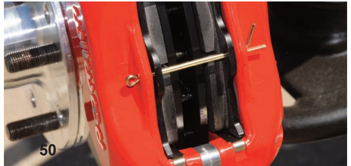
The brake pads are secured into the caliper with this long cotter key.
