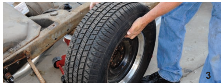
After the lug nuts were disconnected, the tires and wheels were removed from the chassis.
