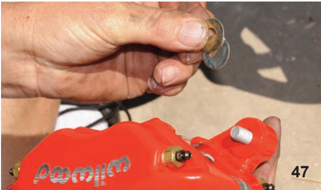
The bolt was placed through the caliper and then it was loaded with two shims. This was done on the top and bottom hole.
