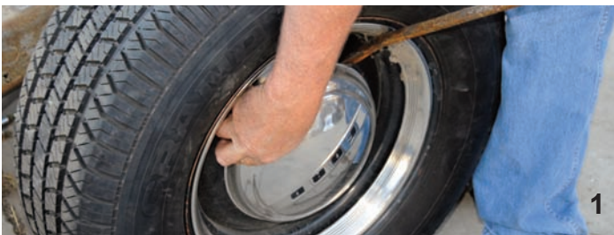
This car is equipped with steel wheels and Ford hubcaps, so the caps had to be removed to access the lug nuts. The caps can be removed by prying the lip up with a large screwdriver.
