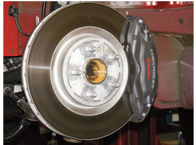
The wheel and tire assembly was removed, revealing the stock brake system and the splined hub assembly. This new Camaro definitely has state-of-the-art styling and engineering.
