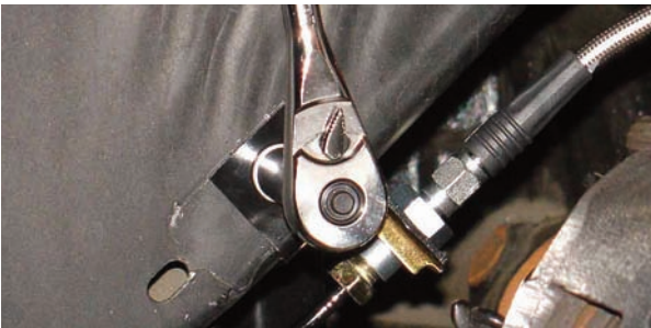
The U-clip was removed from the OEM brake line bracket that is mounted on the inner fender. The bolt and washer holding the bracket on were removed and were retained for reassembly.
