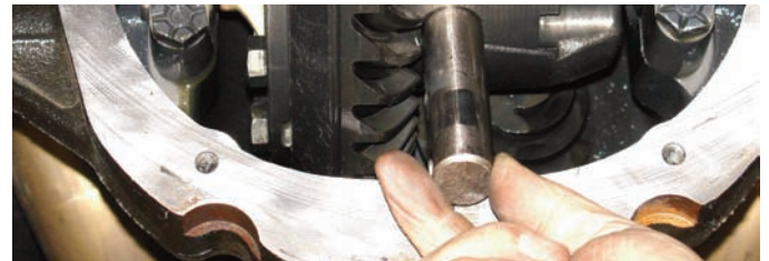
The axle was pressed inward, and then the C-clip was removed from the axle shaft with a drift. After the clip was disconnected, the axle shaft can be removed from the differential. This procedure has to be done on both sides of the differential after the brakes are installed.
