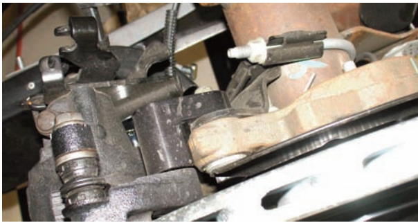
The parking brake cables were disconnected from the OEM calipers.
