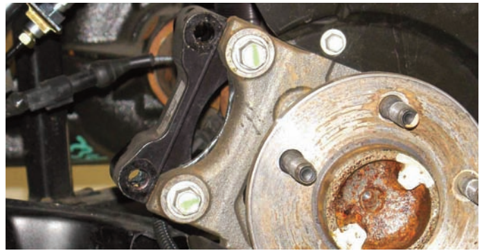
The rotor was tapped with a rubber mallet to release the unit and then it was removed. Here you see the original caliper mounting bracket.
