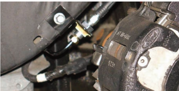
A line wrench was used to disconnect the OEM flex line from the OEM hard line, then the Wilwood stainless steel Flexline (part # 220-9248) was connected to the hard line. The brake line bracket supplied with the Flexline was secured to the same hole used by the OEM bracket using the original bolt and washer. Using a new U-clip, the Flexline was connected to the bracket.
