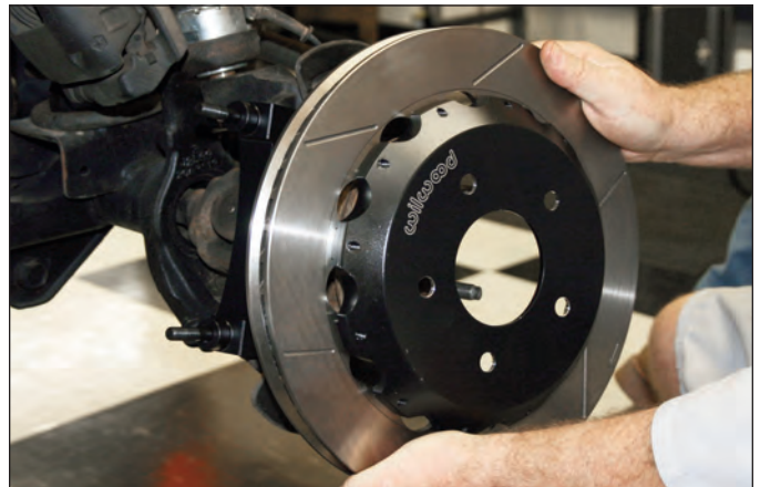
Sequence 11: Install the hat/rotor assembly over the studs on the hub assembly. NOTE: The hat/rotor must fit flush against the axle hub flange or excessive rotor run out may result.
