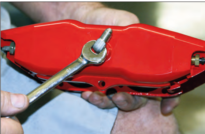
Sequence 15: Remove the protective sticker from the caliper fluid inlet. Coat the inlet fitting with Teflon tape and screw into the caliper with the 90° angle perpendicular to the length of the caliper toward the bleed screws.
