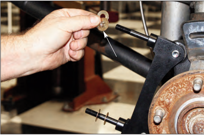
Sequence 13: Lubricate the caliper mounting studs with lightweight oil. Initially place two shim washers on each stud between the bracket and caliper.
