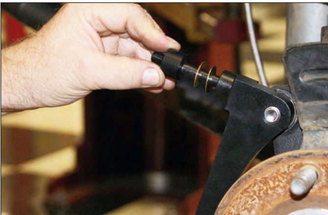
Sequence 14: Slide the caliper spacer over the mounting studs.
