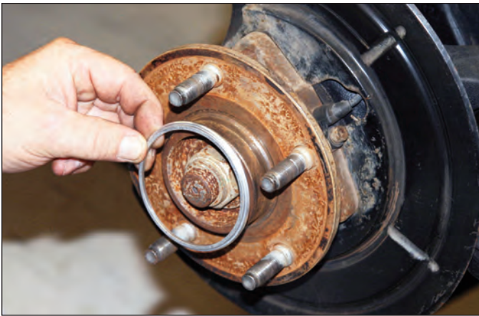
Sequence 7: Install the rotor registration adapter over the hub against the hub face with the larger O.D. facing inward toward the hub face.
