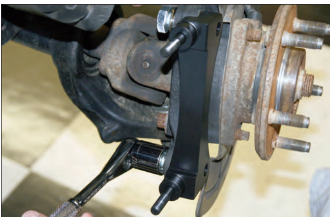
Sequence 9: Attach the Wilwood caliper mounting bracket to the OEM mounting ears on the outboard side. Temporarily tighten the mounting bolts. NOTE: The bracket must fit squarely against the mounting ears. Inspect for interference from casting irregularities, burrs, etc. Grind as necessary. Do not Loctite at this time.
