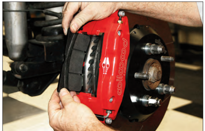
Sequence 18: Having already removed the caliper center bridge pad retainer bolt, nut, and tube from the caliper, insert the brake pads into the caliper with the friction material facing the rotor.
