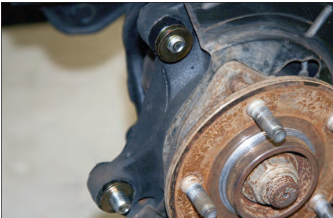
Sequence 8: Slide two caliper mounting bracket bolts through the OEM caliper mounting ears from the inboard side and initially install two shim washers on each bolt.
