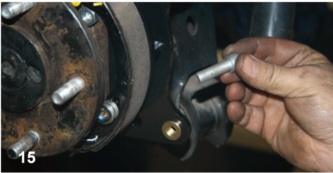
15 Four of these bolts will be used to install the parking brake mechanism and bearing retainer plate to the axle flange. The bolts are installed from the backside of the axle flange as shown here.
