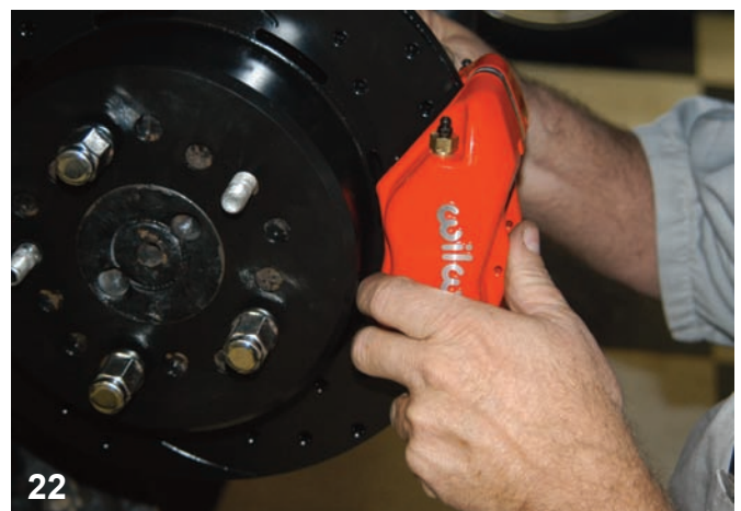
22 The caliper was placed over the rotor and the connections were aligned with the bracket holes. The bolts were connected finger tight to start with.
