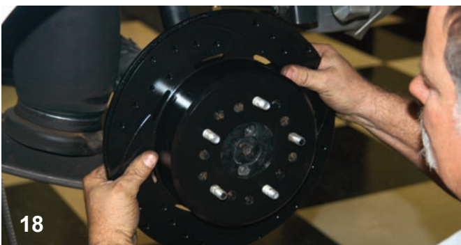
18 The black E-Coated rotor was placed on the studs and was slid back until the opening in the rotor was firmly against the axle flange centering ring. Notice the additional holes that are used to line up with other lug bolt configurations.
