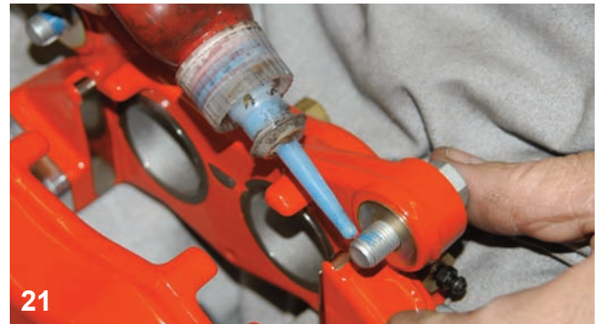
21 It was determined that only one shim washer was required to center the caliper and rotor. Here the attachment bolt was being coated with Loctite prior to installing the caliper.
