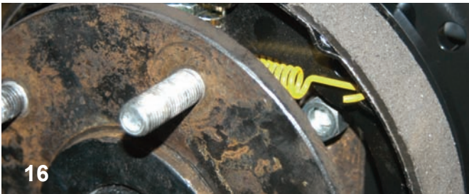
16 Peeking through the opening, you can see the nut on the bolt. Before the nut was installed, a small flat washer was placed on the bolt. This is a tough area to reach, so you will have to be tricky to get the nut connected to the bolt. Tony used a magnet tool to get the parts started.
