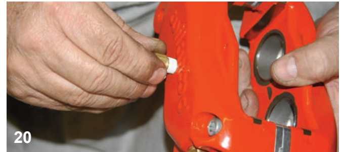
20 The inlet fitting threads were covered with Teflon tape and then the fitting was screwed into the caliper.
