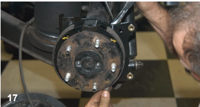
17 All four bolts were tightened with an open-end wrench on the outside and a socket wrench on the backside. The connection should be very tight, so double-check the connection.
