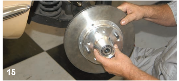
15 The bearings were packed with disc brake bearing grease. The large rear bearing was placed into the hub assembly and the seal was pressed in place. The front bearing was installed in the front of hub and then the hub and rotor were installed on the spindle as seen here.
