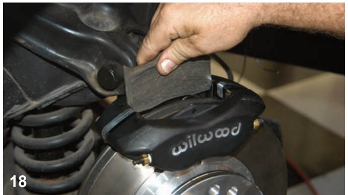
18 The BP-10 Brake pads were installed in the calipers. This is a top loading system that makes brake pad changing easy.
