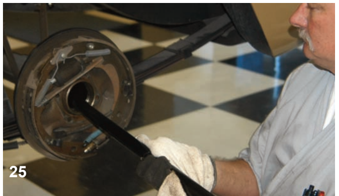
Here Tony is removing the axle assembly. An axle puller may have to be used to break the connection loose.
