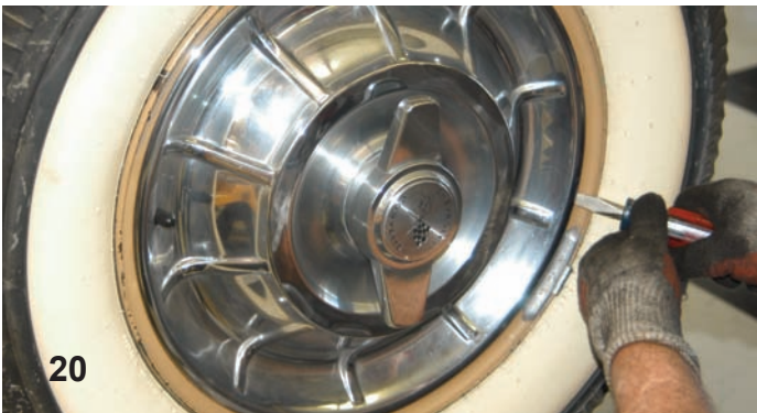
Now we move to the rear suspension. The hubcap was removed by prying the edge up.
