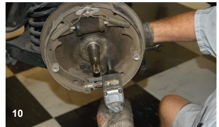
Using an impact gun and a box-end wrench the backing plate nuts and bolts were disconnected.
