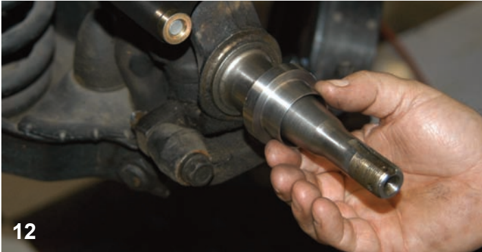
12 Similar to the original hub assembly, the spindle was outfitted with a bearing and seal adapter.
