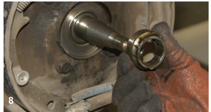
This spindle is equipped with a bearing adapter and spacer. It was removed at this time.
