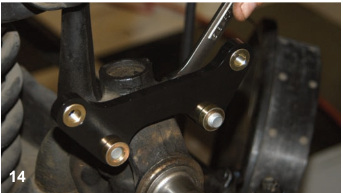
14 The caliper bracket connects to the upper two spindle mounting holes as seen here. On the final assembly, the bolts were coated with Loctite and they were tightened to 35 ft-lbs using a foot-pound torque wrench.
