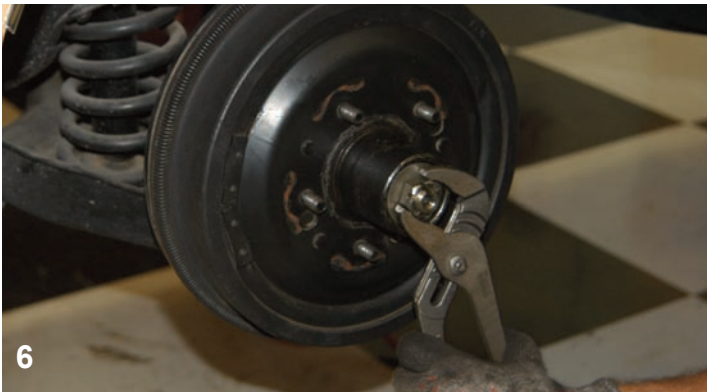
After the cotter key was removed the spindle nut was loosened with the large channel lock pliers. This can also be done using a large crescent wrench.
