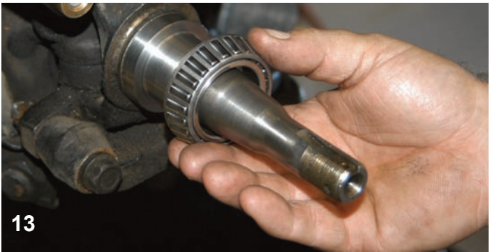
13 Here you can see how the bearing will ride on the front part of the bearing adapter when it is positioned in the hub assembly.
