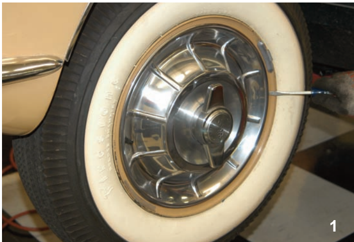
The original Corvette hubcaps were carefully removed by prying the edge up with a screwdriver.
