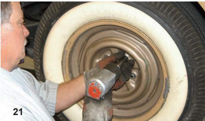
Using an impact gun and the appropriately sized socket, the rear lug nuts were disconnected.
