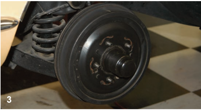
Here is the original Corvette front drum brake assembly. This unit requires removal to install the disc brakes, so hang on it if you ever decide to do a perfect restoration.
