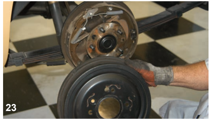
The brake drum was removed, exposing the brake system and backing plate.
