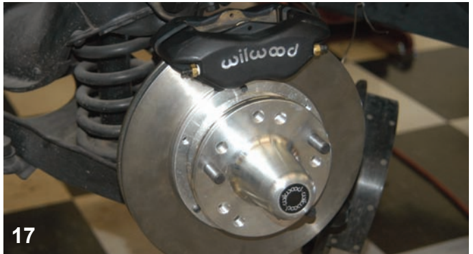
17 The caliper was installed over the rotor, the holes were lined up with the bracket, and then the bolts were installed.
