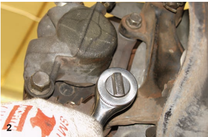
Using a socket wrench and the appropriate size socket, the original caliper bolts were disconnected and the caliper was removed.
