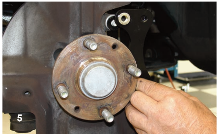
Being careful to keep the bolts in place, the Wilwood caliper bracket was held up to the ears and the bolts were installed by hand. When the bolts were started they were tightened with a socket wrench.
