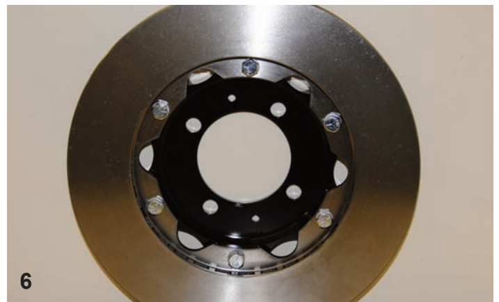
The aluminum rotor adapter was bolted to the rotor using the bolts and washers in the kit. The bolts should be coated with Loctite 271 and then they should be tightened to 85 in-lbs using an inch-pound torque wrench. Using the information in the instruction sheet, the bolts can be safety wired for extra protection
