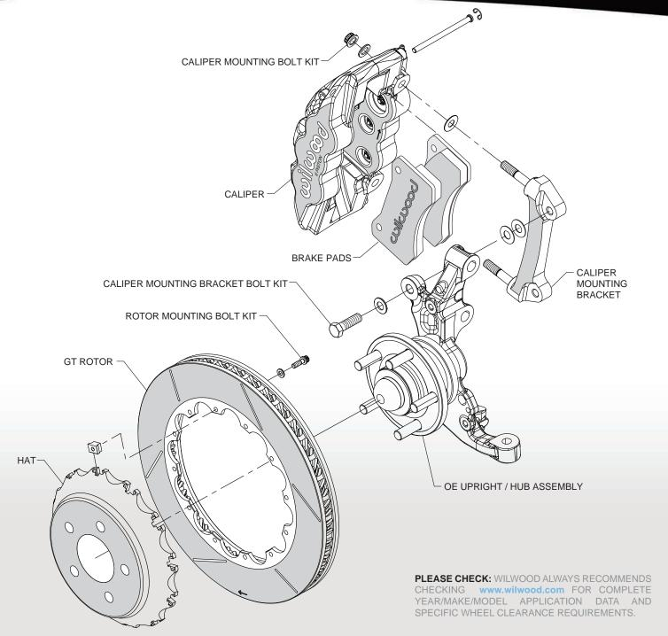
Figure 1. Typical Installation Diagram, Front Kit Shown
