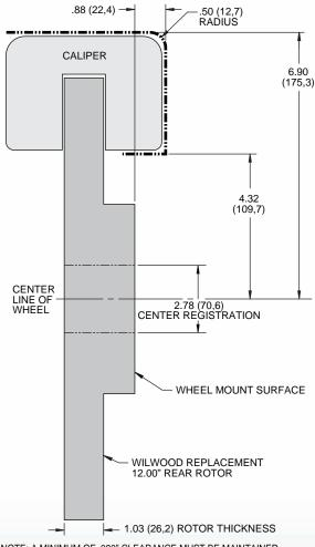
NOTE: A MINIMUM OF .080" CLEARANCE MUST BE MAINTAINED BETWEEN THE WHEEL AND THE CALIPER IN ALL AREAS. THE BACKDROP CLEARANCE OF .88" AND INTERNAL WHEEL RADIUS CLEARANCE OF 6.90" EXCEED THOSE REQUIREMENTS
