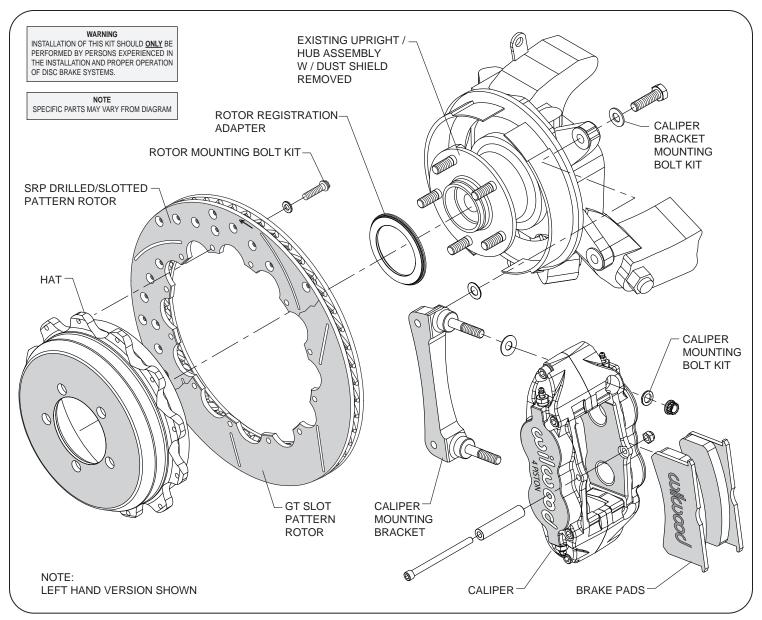
Typical Installation Diagram (2008-2012 Subaru WRX Kit Shown)
