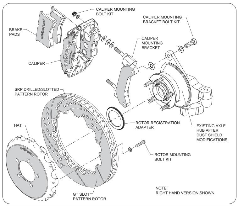
Typical Installation Diagram (FNSL6R 13.06" Kit Shown)
