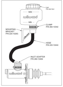
Figure 2. Remote Mounted Master Cylinder
