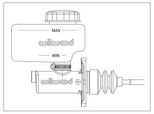
Figure 1. Direct Mounted Master Cylinder
