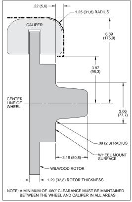
Figure 2. Wheel Clearance Diagram
