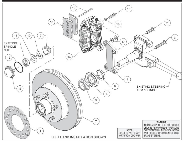
Figure 1. Typical Installation Configuration
