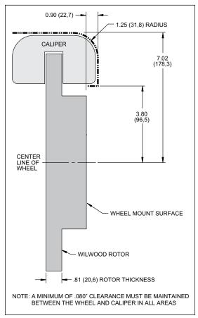
Figure 2. Wheel Clearance Diagram
