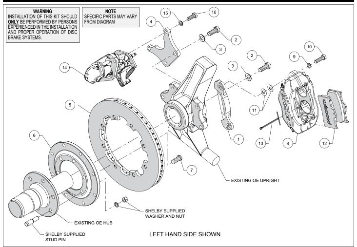
Figure 1. Typical Installation Configuration
