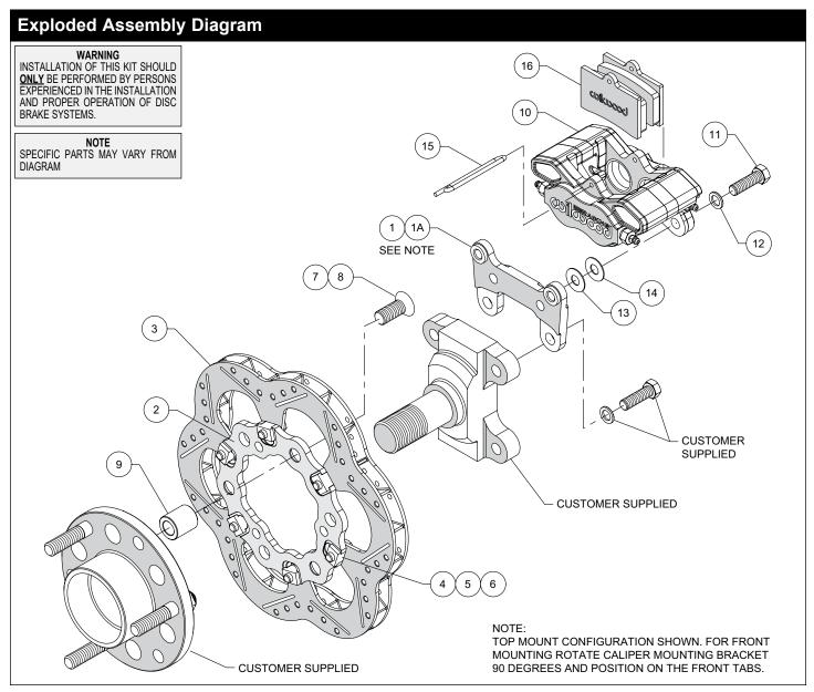
Figure 1. Typical Installation Configuration
