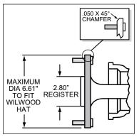
Figure 3. Axle Flange Maximum Dimension
