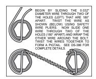
Figure 4. Safety Wire Diagram
