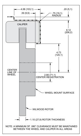
Figure 2. Wheel Clearance Diagram
