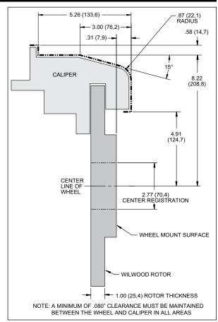
Figure 2. Wheel Clearance Diagram
