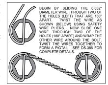
Figure 3. Safety Wire Diagram
