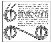
Figure 2. Safety Wire Diagram
