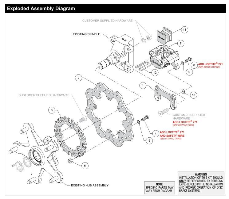
Figure 1. Typical Installation Configuration
